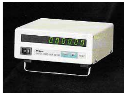
The Nikon TC-101 interpolator with digital read-out
