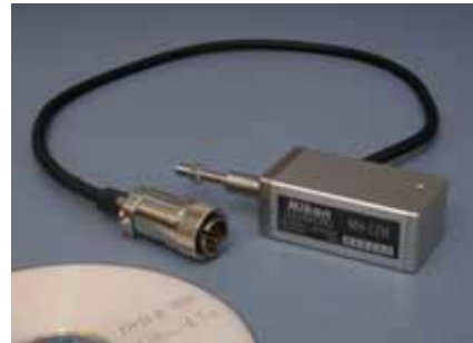
Nikon's compact lightweight MH-12M DigiMicro encoder head
