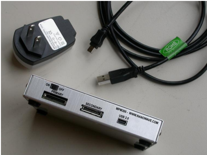
Figure 8 – MPM300 with cable, and wall USB power supply. Enclosure design may vary.
