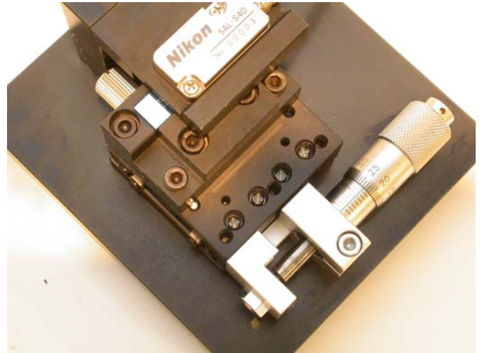
Figure 4 –Example application using Nikon SAL-S40N absolute linear encoder with a micrometer stage.
